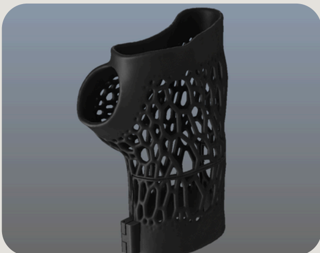
Solidworks model based on Meshmixer data
